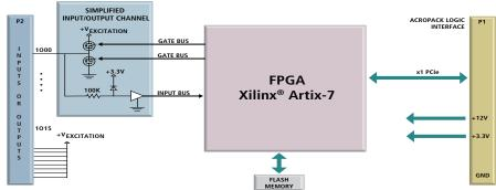
16 Digital I/O Channels ◆ High impedance ◆ PCIe Bus Interface
