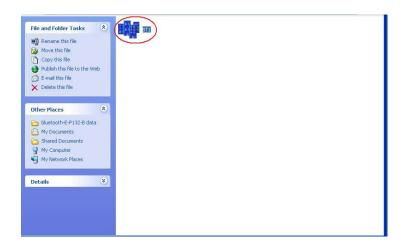
When setting up the BTS-1000A adapter for the first time, you have to install the BT RS232 Config Tool utility software in your computer first which is an executable program in Windows 32-bit environments. The config tool is used to detect and setup the BTS-1000A.
