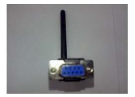
Connect the serial I/O RS-232 connector into devices like computers and other serial devices. (RS-232 RX/TX has been CROSSED OVER)
