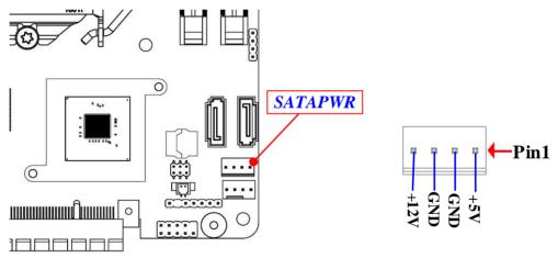
**Warning:** Make sure that Pin-1 of compatible SATA Power connector is inserted into corresponding Pin-1 of **SATAPWR** connector to avoid possible damage to the board and hard disk drive!
