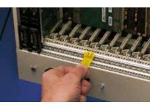
For simple assembly of keys. Up to 3 coding keys may be fitted simultaneously. An integral alignment pin makes positioning easier.
