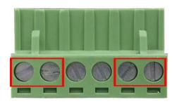
Tighten the wire-clamp screws for preventing the wires from loosing.
