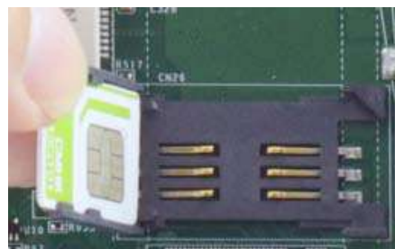
Insert Mini-SIM card with pins facing up
