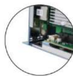
Make sure both cards are inserted into their notches and secured with screws.
