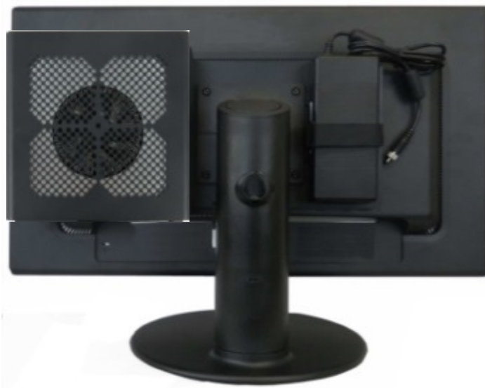
Figure 34: Installed VESA 100 Mount Assembly with VESA Stand Monitor
