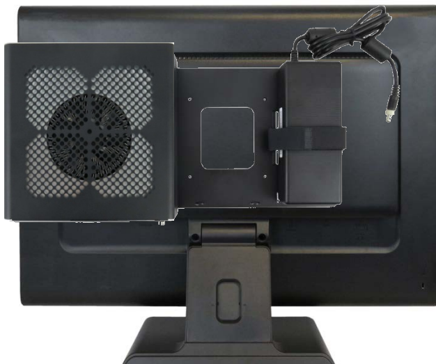
Figure 32: Installed VESA 100 Mount Assembly on a non-VESA Stand Monitor
