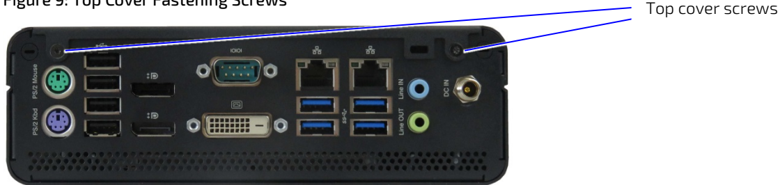
Figure 9: Top Cover Fastening Screws
